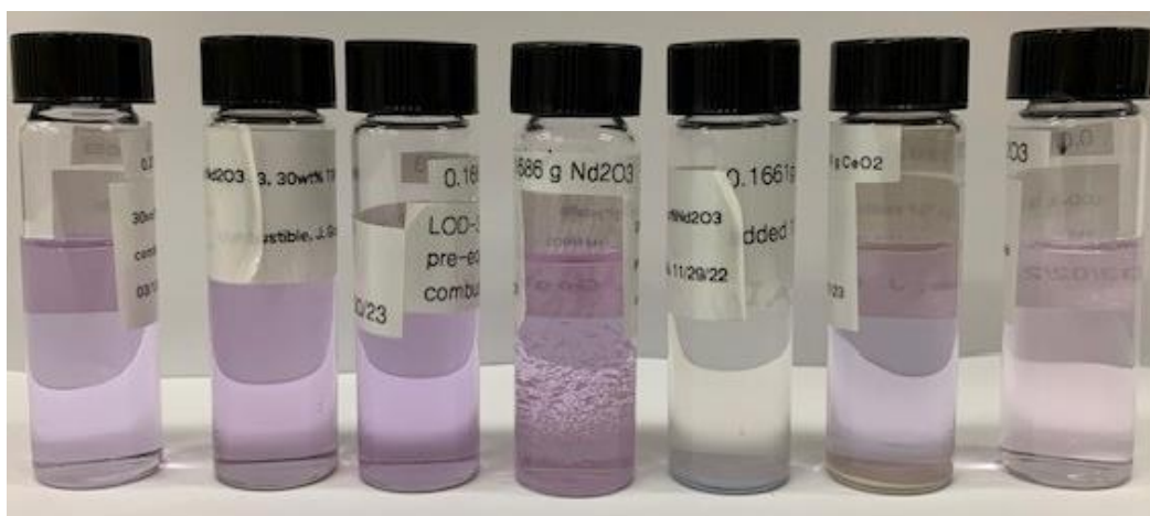
Figure 1: Neodymium in 30 vol % TBP-paraffin (Vials 1-6) and Nitric Acid (Vial 7)
