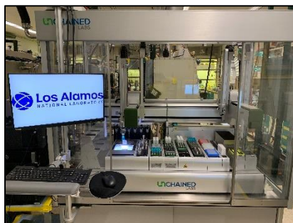
Fig 1. LANL Super Separator – an automation system for high-throughput separation.
