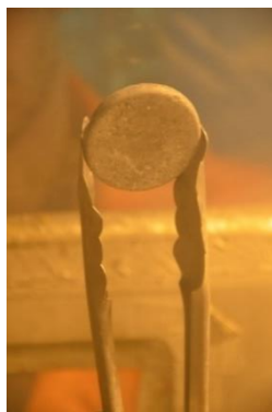
Figure 1. Plutonium metal button product from modified DOR process.
